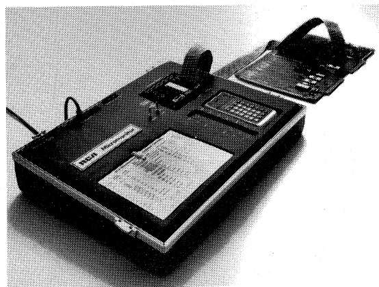
Fig. 2 — Use of Micromonitor as a prototype hardware and software debugging tool with COSMAC Developmental System II CDP18S005.
